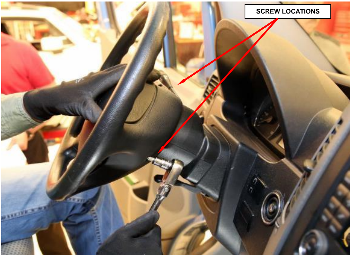
Figure 3 - Driver Airbag Screws
